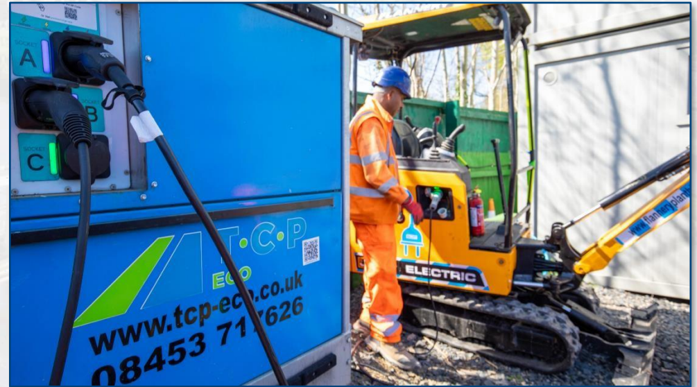
While working at Bewdley in Worcestershire, Jackson tested the use of solar photovoltaic (PV) in charging electric plant. These projects are part of a one-year trial made possible through funding from the EA's Net Zero Carbon Innovation Pathway Fund.
